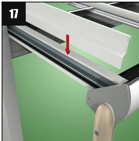
17 Complete the installation of the cloaking trim.
